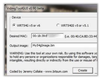
the vximgtoolgui application and filling in the MAC address I wrote down from underneath my router, and pointing the app at a place to drop the resulting .bin file.
